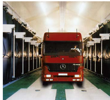
A testing system for performing alternating tests for corrosion testing in the automobile industry
