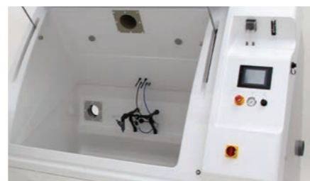
3. The Atmosfär chamber is now ready for other types of corrosion test.
